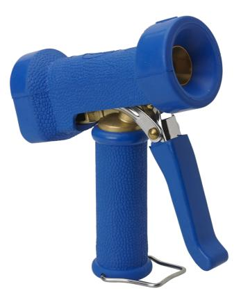
The Heavy Duty Water Gun is suitable for cleaning floors and machinery, and for rinsing off work surfaces and walls after chemical foaming. Determine the jet pattern by squeezing the rubber insulated trigger. Adjust the water jet with a screw at the end of the gun. An arrow on the gun shows the water spray direction. Use 0712 1/2" or 0715 3/4" hose nipples, which can be screwed into the bottom of the gun. You need one of these nipples to connect a hose to the gun.
