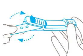
Reverse or replace the blade. Make sure you place the blade **exactly on the locating lobes**.
