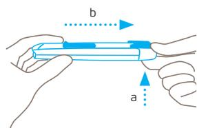
Press the blade change button **pushing up from below** and remove the plastic insert from the rear of the handle.
